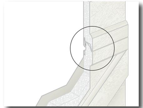
The pinch resistant profiles of top and bottom rails are molded to the section in a one piece construction.
